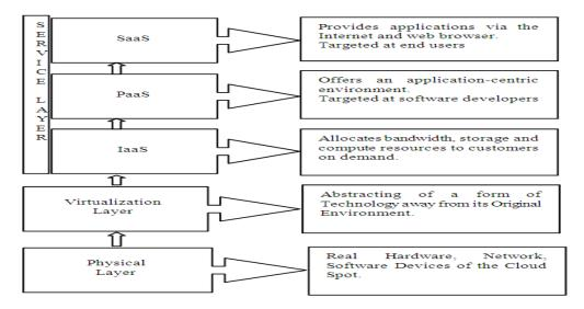
Figure 1. Layered Cloud Architecture
